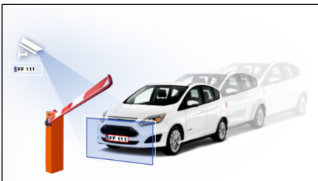
ANPR Camera based parking system which recognition only the authorized vehicles to enter into the premises
